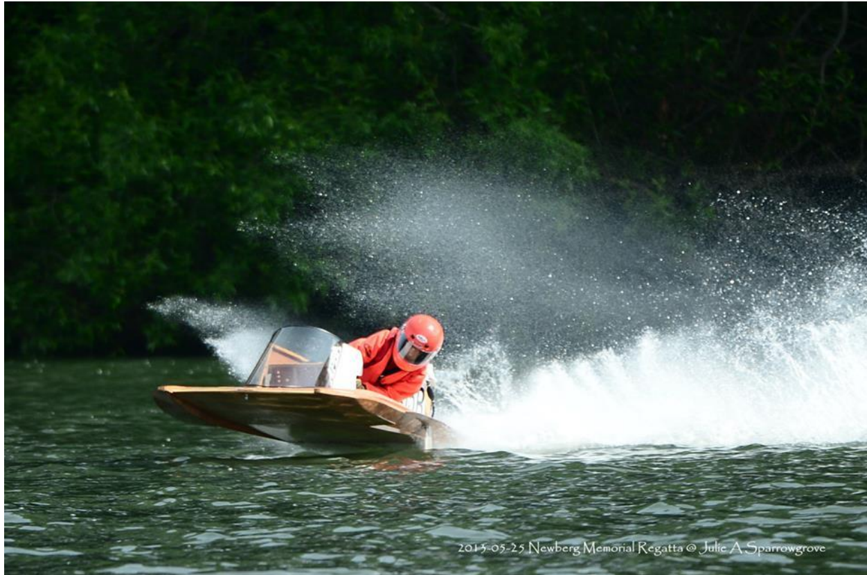
Figure 3. A good example of running a little TOO high. This driver was real wet shortly after the photo was taken.
